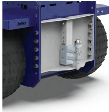
Multifunction hitch ball / drop pin
