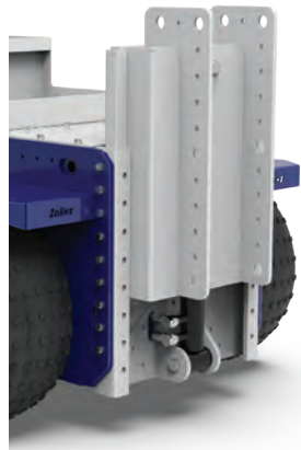
Drop pin hitch Ø35 / 40 / 50 mm
