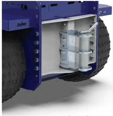
Drop pin hitch Ø35 / 40 / 50 mm
